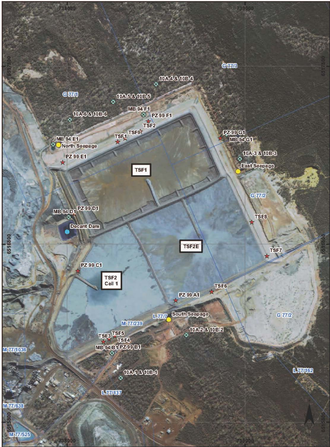
TSF Monitoring Locations Marvel Loch (Attachment 1) Date : 30 August 2010 Drawn by : A Fisher Ref : M:\02.User_Projects\2.3.Regional\Western_Aust\Southern Cross\Environmental\Monitoring\100830_Marvel Loch TSF Bore Monitoring Locations.mxd 0 70 140 280 420 560 Meters Projection : Map Grid of Australia Zone 50 Datum : Geocentric Datum of Australia 1994 (GDA94) St Barbara Limited
